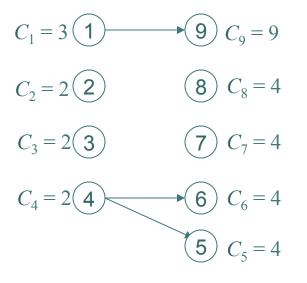
9 tasks with precedences and the shown execution times, where lower numbered tasks have higher priority than higher numbered tasks. Priority-based 3 processor schedule:
