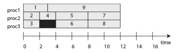
The priority-based schedule with four processors has a longer execution time.
