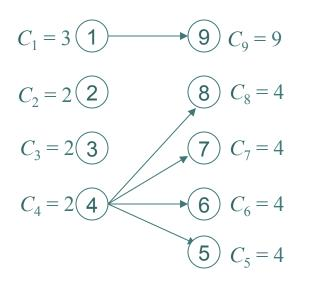
9 tasks with precedences and the shown execution times, where lower numbered tasks have higher priority than higher numbered tasks. Priority-based 3 processor schedule:
