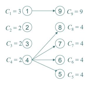
Priority-based scheduling is "greedy." A smarter scheduler for this example could hold off scheduling 5, 6, or 7, leaving a processor idle for one time unit. 9 tasks with precedences and the shown execution times, where lower numbered tasks have higher priority than higher numbered tasks. Priority-based 3 processor schedule:
