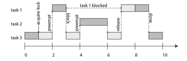
Task 1 has highest priority, task 3 lowest. Task 3 acquires a lock on a shared object, entering a critical section. It gets preempted by task 1, which then tries to acquire the lock and blocks. Task 2 preempts task 3 at time 4, keeping the higher priority task 1 blocked for an unbounded amount of time. In effect, the priorities of tasks 1 and 2 get inverted, since task 2 can keep task 1 waiting arbitrarily long.
