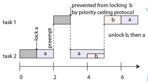
In this version, locks a and b have priority ceilings equal to the priority of task 1. At time 3, task 1 attempts to lock *b*, but it can't because task 2 currently holds lock *a*, which has priority ceiling equal to the priority of task 1. #include <pthread.h>
