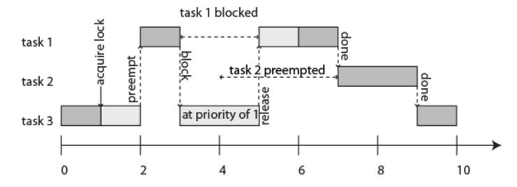
Task 1 has highest priority, task 3 lowest. Task 3 acquires a lock on a shared object, entering a critical section. It gets preempted by task 1, which then tries to acquire the lock and blocks. Task 3 inherits the priority of task 1, preventing preemption by task 2.
