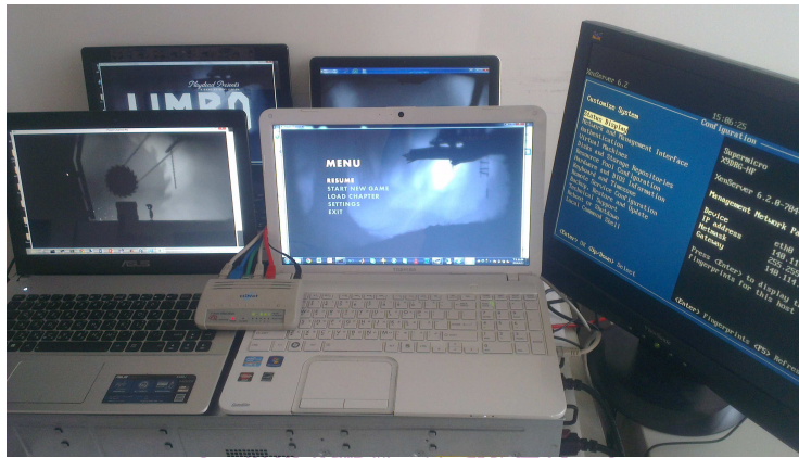
Figure 8.1: Our testbed with a cloud game server (right) and four game clients (left), connected by a Fast Ethernet switch (middle).
