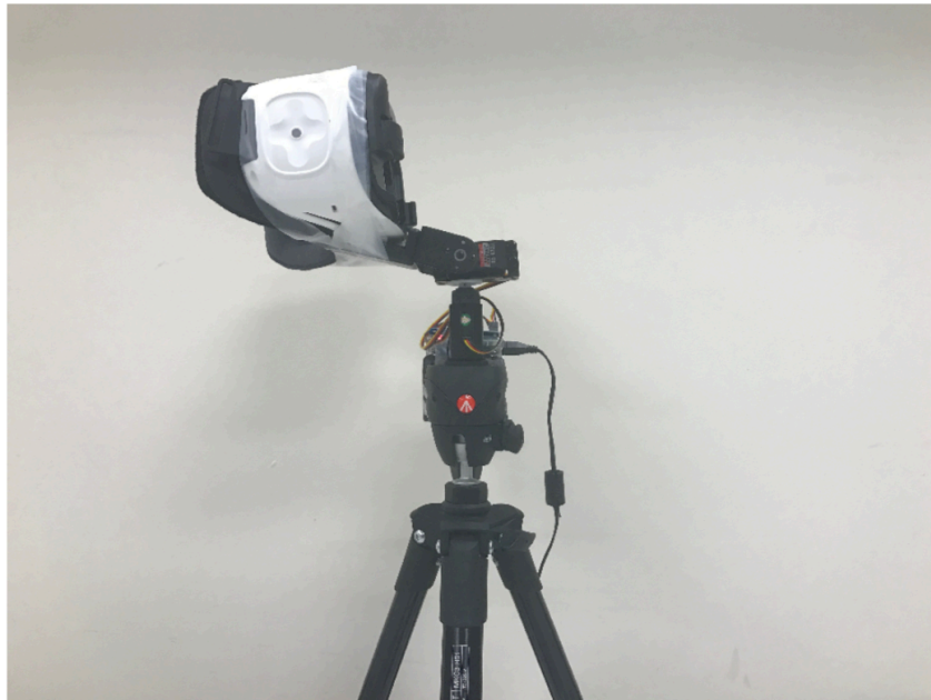
Figure 8: Our VR testbed consists of a GearVR, an S7, a Pan/Tilt mount, a 3D-printed holder for the mount, a Raspberry Pi to accurately control the mount's motion, and a tripod for stabilizing the test instruments.
