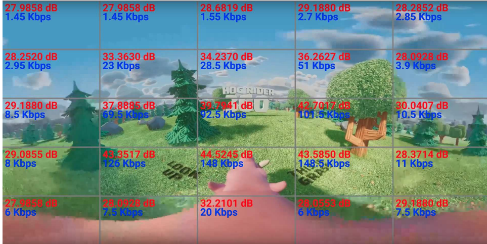
Figure 3.4: A sample clip of TR approach in equirectangular projection.
