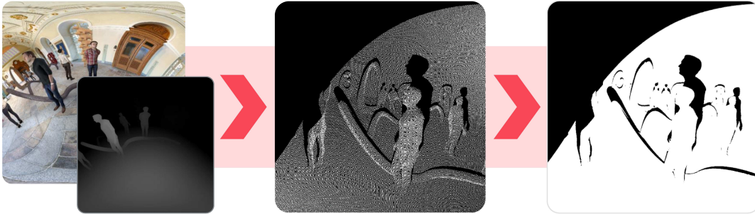
Figure 4.2: Mask generation process in the mask generator component, including two steps of process: 3D warping and hole filtering.
