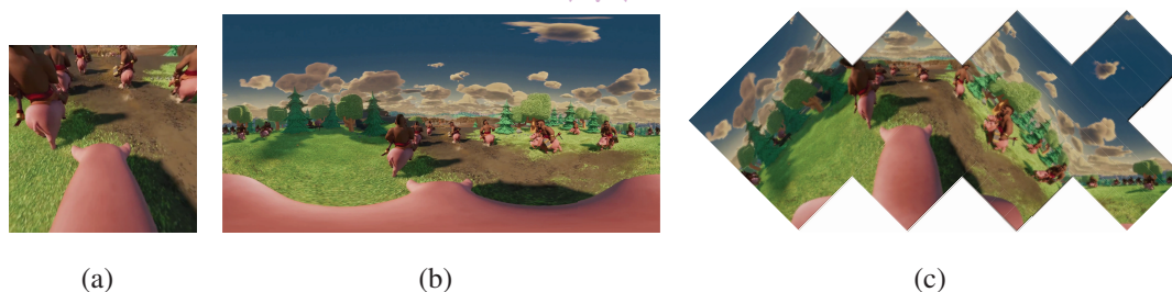
Figure 3.1: A sample image: (a) seen in HMDs; distorted images due to: (b) equirectangular projection and (c) rhombic dodecahedron projection.
