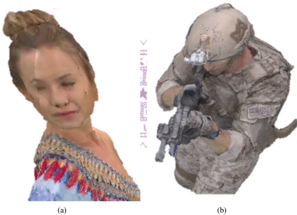
Figure 8.1: Less than perfect concealed point clouds due to: (a) extrusion of facial expression and (b) rotation of the rifle.
