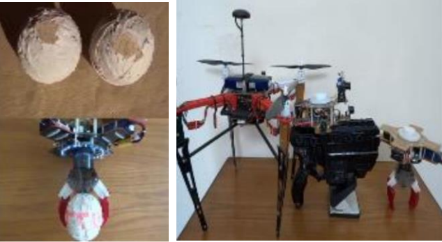
Fire extinguishing system: quadrotor, gun, robot, and extinguishing balls. [IJIGSP'18]
