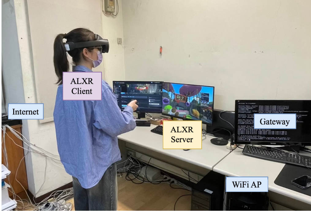
Figure 5.3: Our developed cloud VR gaming testbed photo.
